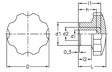
$$\begin{array}{lll} D & = 85 \\ d1 & = 32 \\ d2 & = 20 \\ d & H9 = 8 \\ h & = 26 \\ L & = 49 \\ l1 & = 35 \\ l2 & = 21 \\ \end{array}$$
